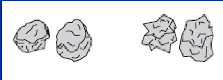
subangular (left) and angular blocky
